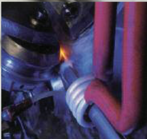
The edges of the formed tube are high frequency electric-resistance welded, providing a smooth contour and maintaining tight tolerances
